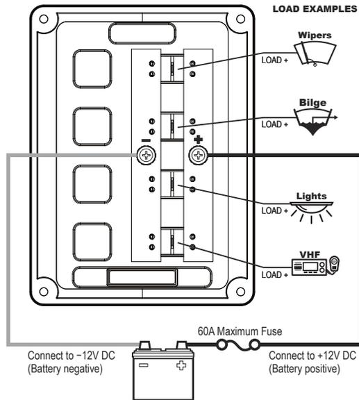
LOAD = Any appliance consuming power, i.e... stereo, lights, horn, etc.
