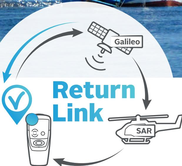
Return Link's blue light confirms distress signal has been detected and independently located.
