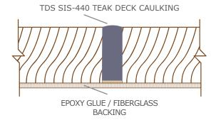
\* Use of polyurethane bond breaker tape aids to achieve 2-sided adhesion. The bottom of the caulk seam should be able to move at the base of the seam, as the deck flexes and works.
