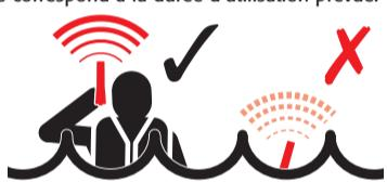
The S10 must always be kept above water when activated, as direct contact with the sea will severely reduce the transmission range.
