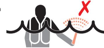
For optimum transmission, the S10 must be held upright when activated.
